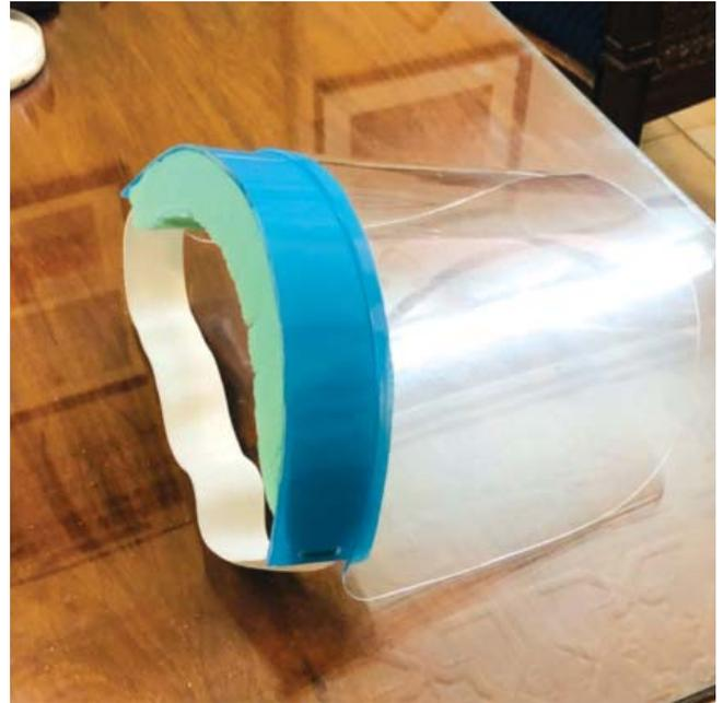
**Figure-1:** In-house faceshield re-useable made from local resources (acrylic sheet plus foam and elastic). Approximate cost Rs 500.
