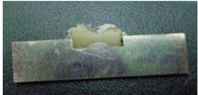
Figure-2: Specimens in the mould after curing.
