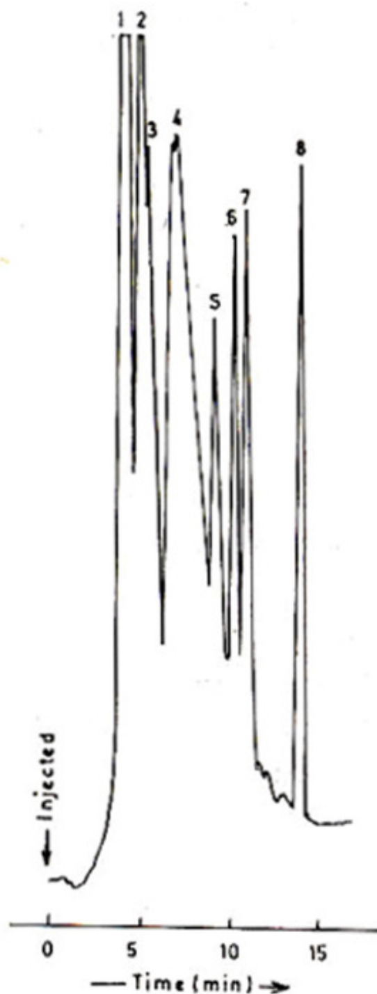
Figure 4. Chromatogram of dichloromethane extract of urine doped with testosterone esters standard peak identification (1, 2, 3, 4 = natural urine components), 5 = T. propionate, 6 = T. isocaproate, 7 = T. phenyl propionate, 8 = T. decanoate chromatographic conditions same as in Figure 3.
