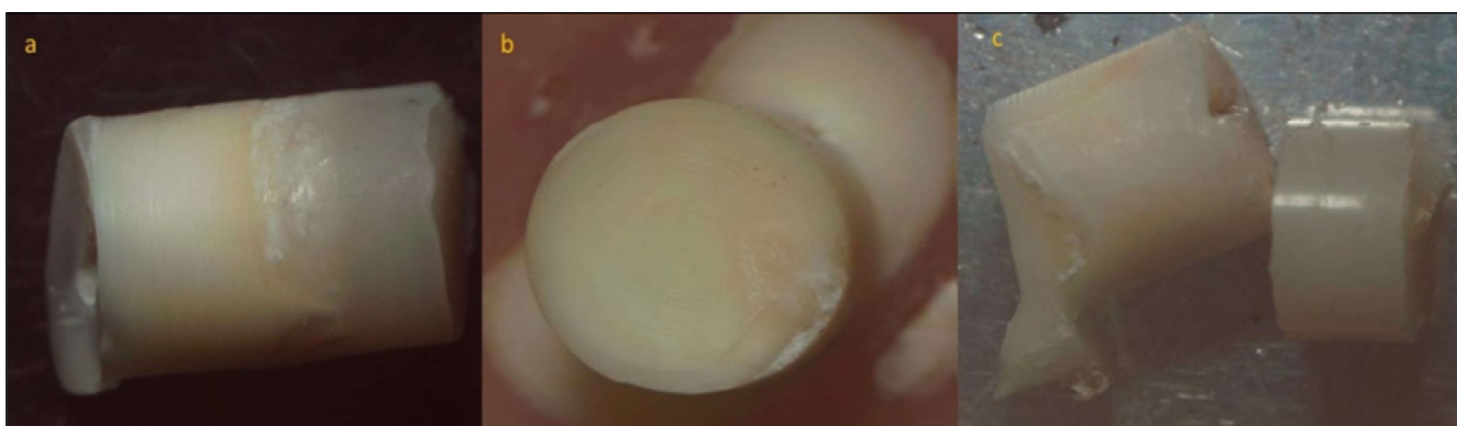
Figure-2: Fracture pattern behaviour of (a) control, (b) Proanthocyanadine (PA), and (c) Genepin (GE).
